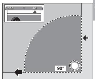
Align the right stop to the watering area by adjusting the watering arc angle.
