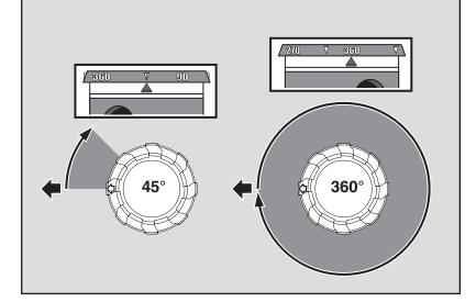
Use the sprinkler tool or a screwdriver to adjust the right stop of the watering arc. Rotate clockwise to increase or counter-clockwise to decrease.
