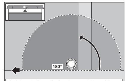
The left stop indicates the fix point or  $0^{\circ}$  of the arc. The arc angle will determine the right stop of the watering arc.
