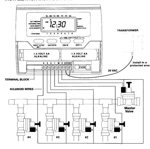
Remove the lower cover. Place the unit on the wall using one slot and one fixed hole inside the battery slot. Connect the solenoid wires to the terminal block. One wire from each solenoid should be connected to "C"-Common. The other wire from each solenoid connects to its respective number on the terminal block. Connect the transformer wires to the terminal block marked 24VAC.
